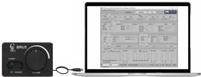
Figure 1: Connect the BRU5 to a personal computer or laptop and ensure that you have installed the ACP Workbench application.
